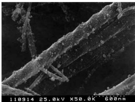
Figure 4. SEM image of the silica structure prepared by transcription of helically bundled 1 as a template (before calcination).
